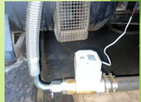
Electronic ball valve (Solenoid valve)
