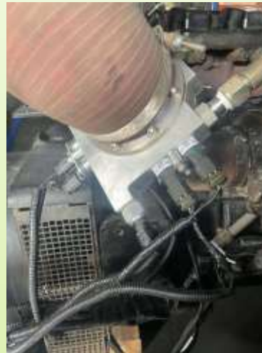
Rail pressure & temperature sensor and CNG injectors
