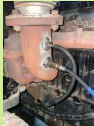
Exhaust temperature & Oxygen sensor
