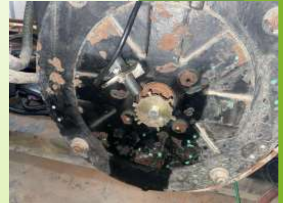
Trigger wheel and crank position sensor
